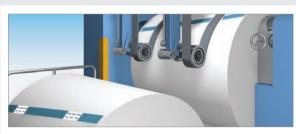
Belt-driven machines present a unique set of demands for a splicing tape: the tension differences between the belt-path and the rest of the web during the splicing process can lead to tears and creases in the paper.
